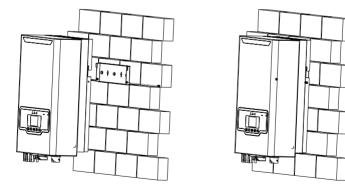
Figure 4.6 Mount the Inverter
