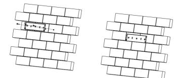
Figure 4.5 Mount the Rear Panel
