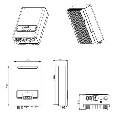
Figure 3.2 Dimensions of Suntrack Plus 4K/5K/6K/8K/10K
