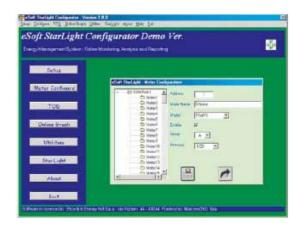
The second step: from simple tree, and the selected instrument model like the instrument used communication protocol name, to distinguish the load area and cost. Ready to proceed! Just a few clicks of the mouse you can configure the system.
