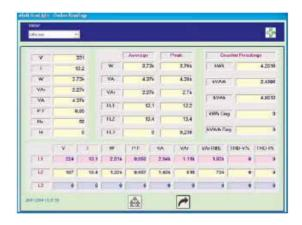
"Active data" window displays all of the real-time measurements; There are two different display modes: 1) Comprising a read page from all measured values of the measured loads selected. Synthesis relevant set of readings separable four columns: the three-phase values, average and peak power measured value, with L1-L2-L3 Value.
