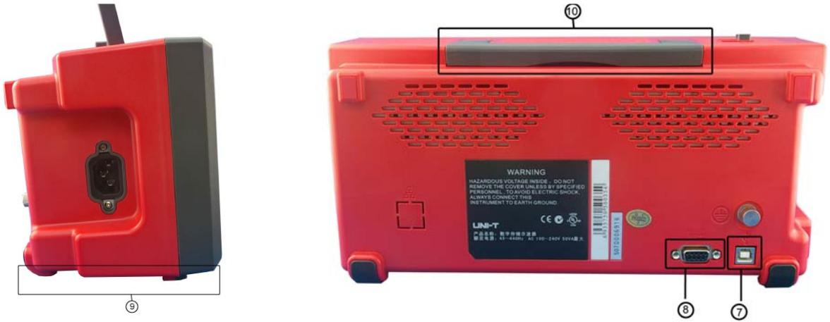
⑦ & ⑧, USB Port and RS-232 Port Combined with Digital Oscilloscope Virtual Panel for PC Connectivity
