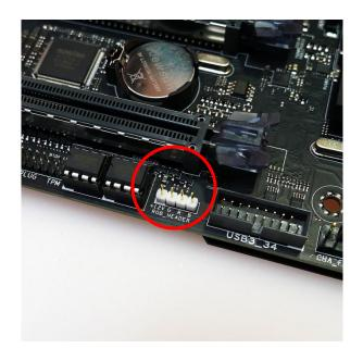
• 1) Require motherboard with RGB header to enable RGB lighting
