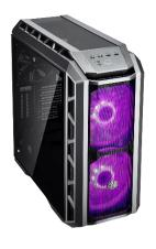
Clear View Inside – The MasterCase H500P Mesh has a light grey tinted tempered glass side panel and a plastic top cover, making it ideal for showcasing your build with (RGB) lighting.
