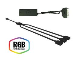
RGB controller and 1 to 3 Splitter Cable for RGB LED Fans – The included RGB controller can be connected to the Reset Switch to manage the lighting of the two 200mm RGB fans. Also the RGB Connector Splitter and 4 pin male to male adapters are included
